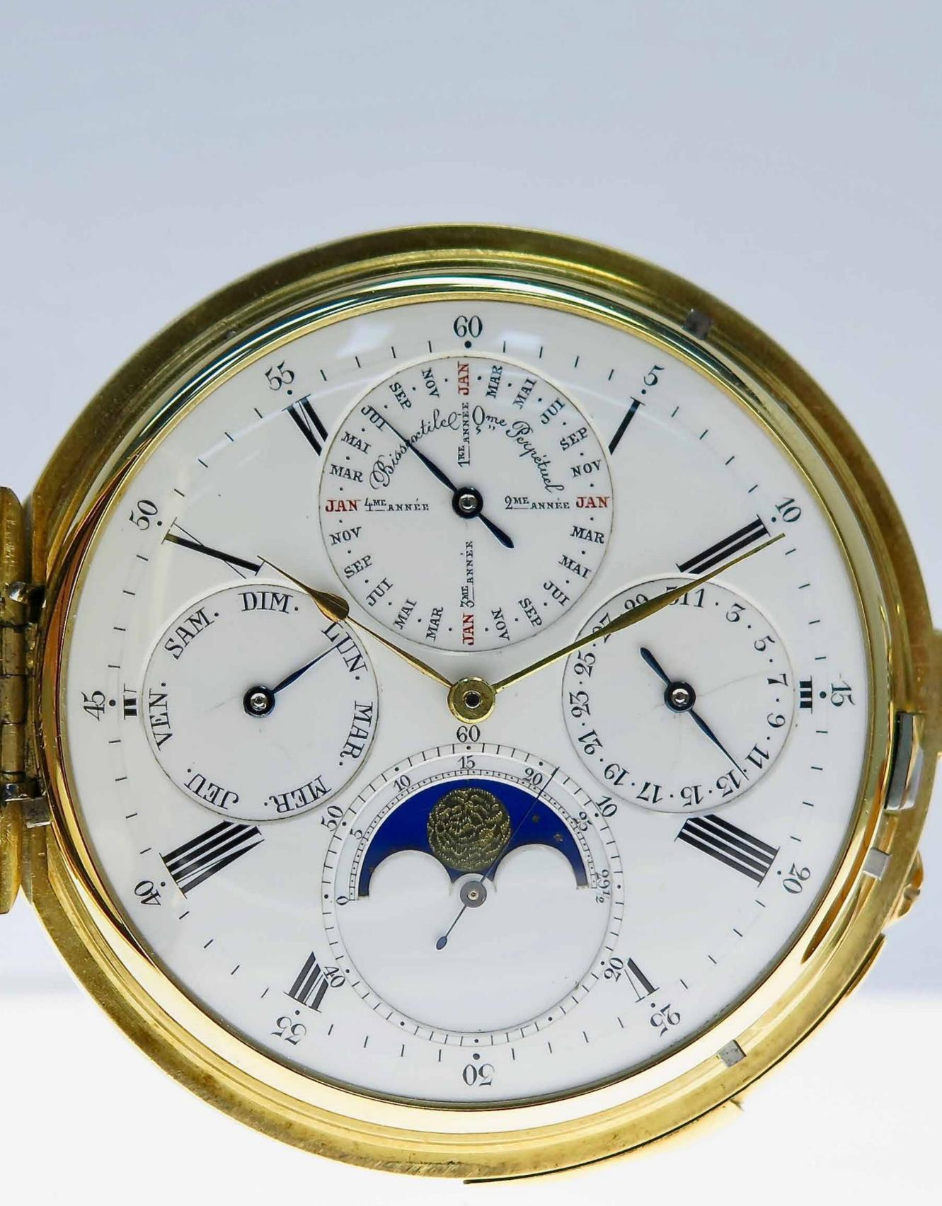
The layout for the perpetual calendar is classical and has been repeated countless times during watchmaking history, for both design and technical reasons. The months set at 12 o'clock, the day at 9 and date at 3 o'clock. The moon phases disc set at 6 o'clock with the seconds passing through the centre.
